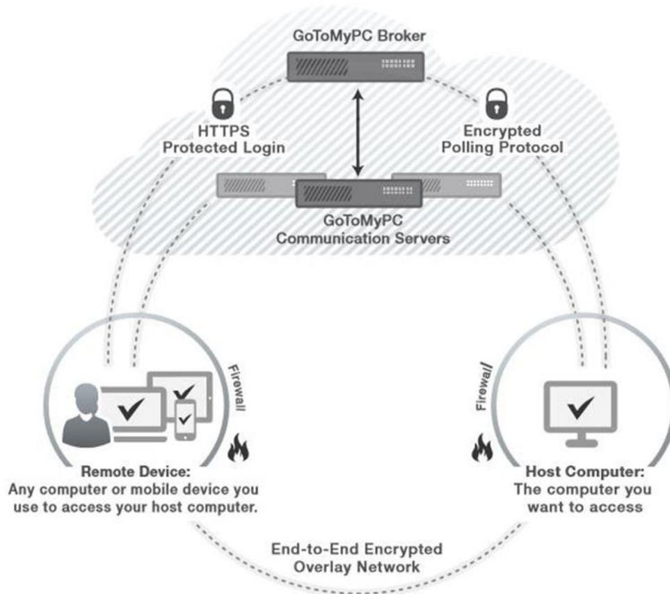
The infrastructure is designed in a manner intended to be both robust and secure. Redundant routers, switches, server clusters and backup systems are designed and employed to ensure high availability. For scalability and reliability, switches transparently distribute incoming requests among web servers. For the purposes of ensuring optimal performance, the GoToMyPC broker load balances the client/server sessions across geographically distributed communication servers.
