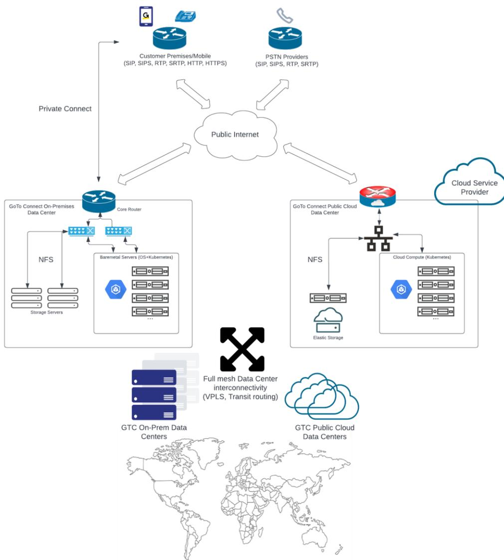
Figure 1: GoTo Connect Architecture
