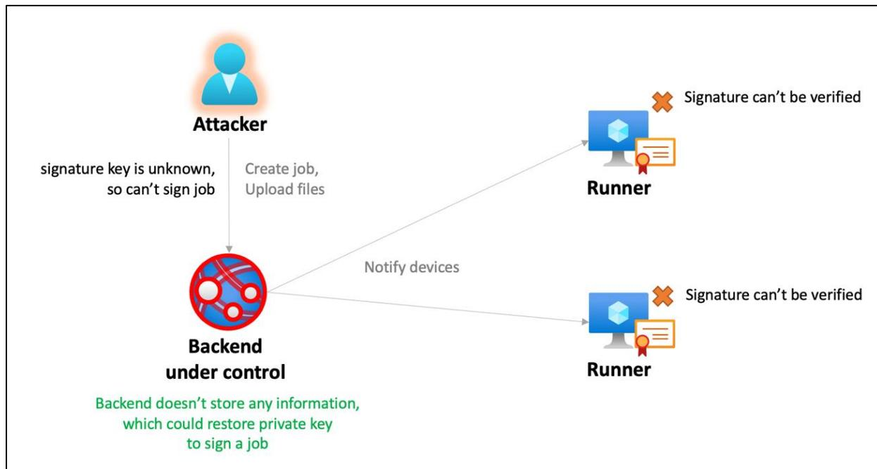
Figure 4. Compromised Backend within a Zero Trust Environment
